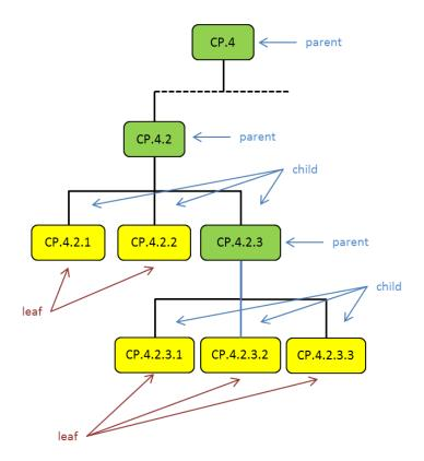
Figure 3 Portion of the Functional Model hierarchical structure
