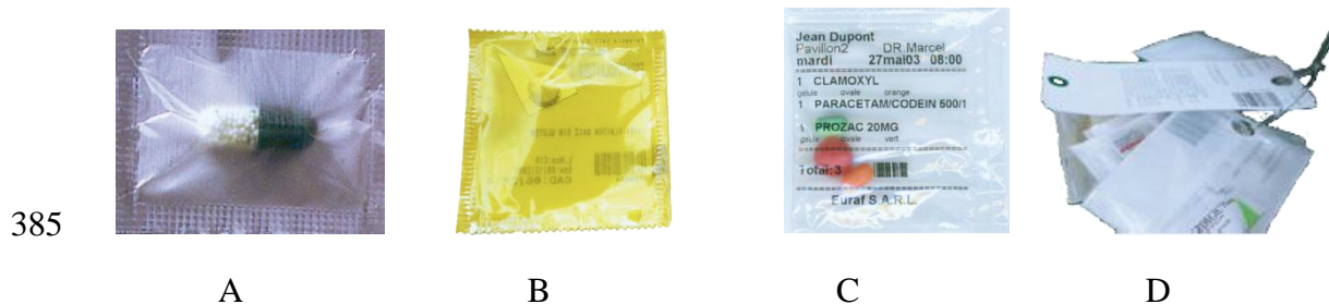
390 Figure 6 – Various logistics objects: A) Primary repackaging B) Unit Dose Overwrapping C) Packaging of an individual dose according to the schedule D) Secondary Packaging of a ring of individual doses. Note that on the packing of individual doses one can see an identifying barcode and a description of its contents. On the label identifying the ring one can see the identifying barcode and the list of individual doses.
