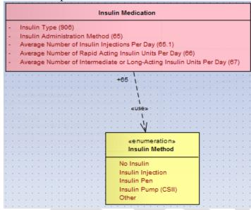
The permissible values are modeled as values (red text) of enumerations (yellow rectangle) in the class diagram. The enumerations are connected to their respective referring attribute (red text inside the pink rectangle) with "use" relationship, drawn as a dashed arrow with a "<<use>>>"
